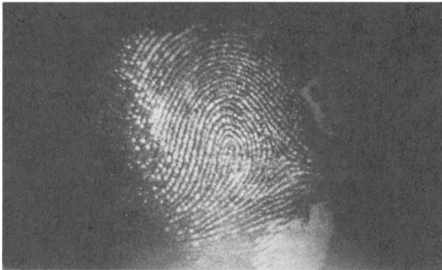
FIG. 2—Latent print on glass dusted with FMP 01/Nile blue and developed by red laser illumination.
