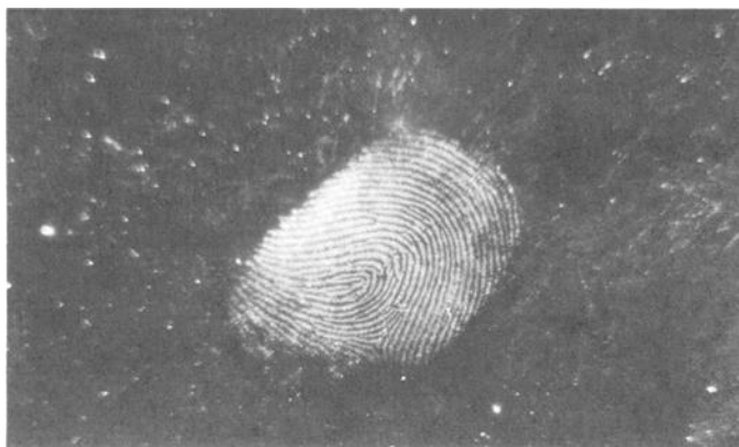
FIG. 1—Latent print on plastic dusted with FMP 01/rhodamine 6G and developed by argon laser illumination.
